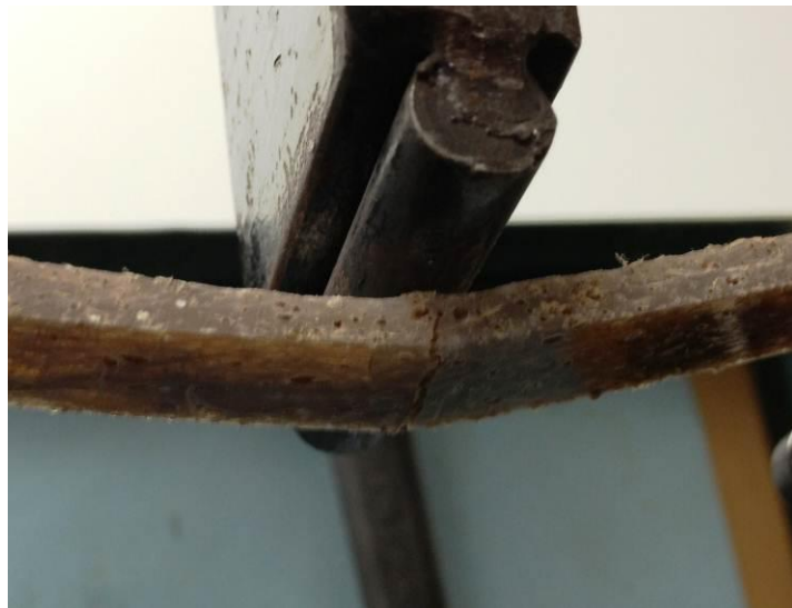
Figure 4. Failure of bamboo composites under bending
