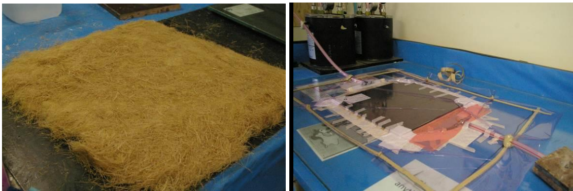
(a) Randomly oriented bamboo fibres (b) Vacuum infused bamboo fibre composites Figure 1. Preparation of bamboo fibre composites
