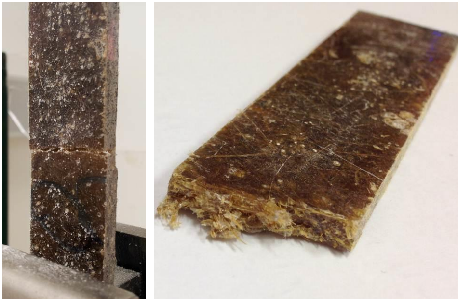
Figure 6. Failure of bamboo composites under tension
