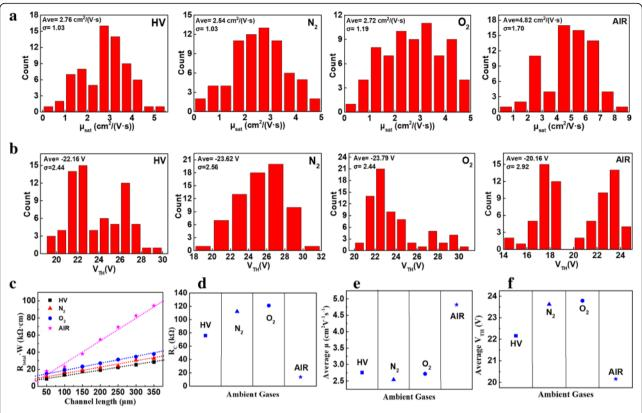
**Fig. 3** (Color online) Statistical histograms of the carrier mobilities (**a**) and threshold voltages (**b**) observed from devices exposed to various test gases. **c** Transmission line model plots with linear fittings of  $R_{\text{total}}$  W and impacts of environmental conditions on contact resistances (**d**), average mobilities (**e**), and average threshold voltages (**f**)
