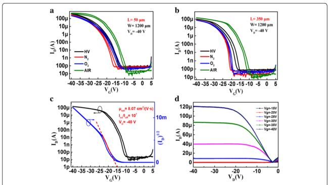
**Fig. 2** (Color online) Typical transfer characteristics of transistors after exposure to various environmental conditions:  $50 \, \mu m$  (**a**) and  $350 \, \mu m$  (**b**) channel lengths. Typical transfer characteristics (**c**) and output characteristics (**d**) of devices with mobilities of 8.07 cm<sup>2</sup> (V s)<sup>-1</sup>,  $I_{on}/I_{off}$  ratios of  $10^7$ , and  $350 \, \mu m$ -long channels
