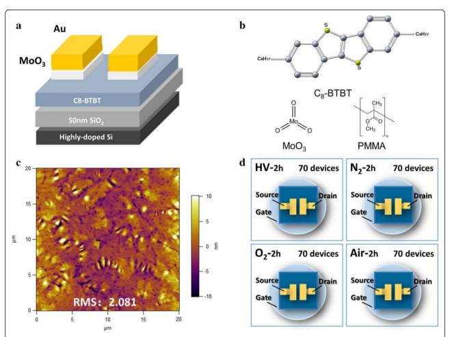
**Fig. 1** (Color online) (**a**) A schematic diagram of the device structure. (**b**) The molecular structures of the C8-BTBT, molybdenum oxide, and PMMA used in the experiment. (**c**) AFM surface morphology image of the C8-BTBT film indicating a small RMS value of 2.08 nm. (**d**) Test procedures used to measure the electrical performance characteristics of 70 units of each device type (high vacuum, nitrogen atmosphere, oxygen atmosphere, and air atmosphere)
