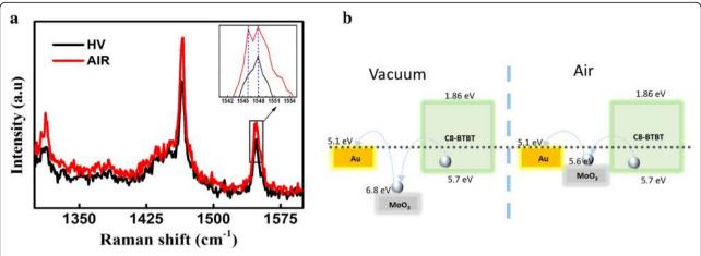
**Fig. 4** (Color online) (a) Raman spectra ( $\lambda_{\rm exc} = 633$  nm) of C8-BTBT thin films in HV and air conditions. The inset shows an enlargement of the area between 1542 and 1554 cm<sup>-1</sup>. (b) Schematic diagrams of work function changes in MoO<sub>x</sub> in HV- and air devices, resulting in the reduction of the barrier height associated with charge injection from the S/D electrode to C8-BTBT
