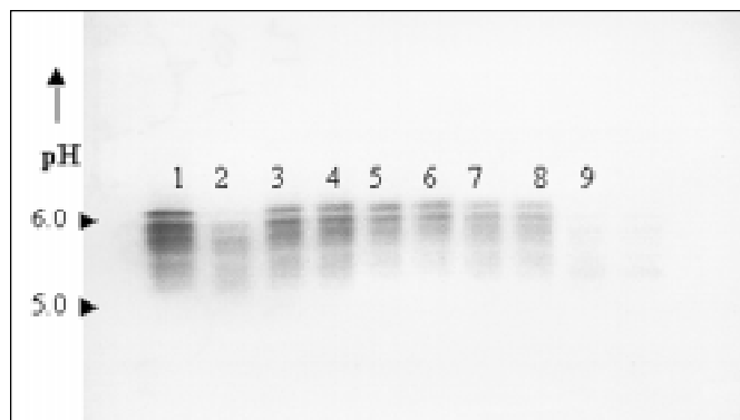
Figure 3—Isoelectric focusing of cantaloupe melon peroxidase. 1 = fresh-cut fruit immediately after processing, 2 = the same fruit after 6 d storage at 4 °C, 3 = fruit dipped in ascorbic acid (1.25 mM) after 2 d storage, 4 = fruit dipped in ascorbic acid immediately after fresh cut processing, 5 = fruit dipped in ascorbic acid (1.25 mM) immediately after fresh cut processing, 6 = fruit dipped in ascorbic acid (2.5 mM) after 2 d, 7 = fruit dipped in ascorbic acid (2.5 mM) after 6 d, 8 = cut fruit after 15 d storage and 9 = fruit dipped in ascorbic acid (2.5 mM) after 15 d storage.
