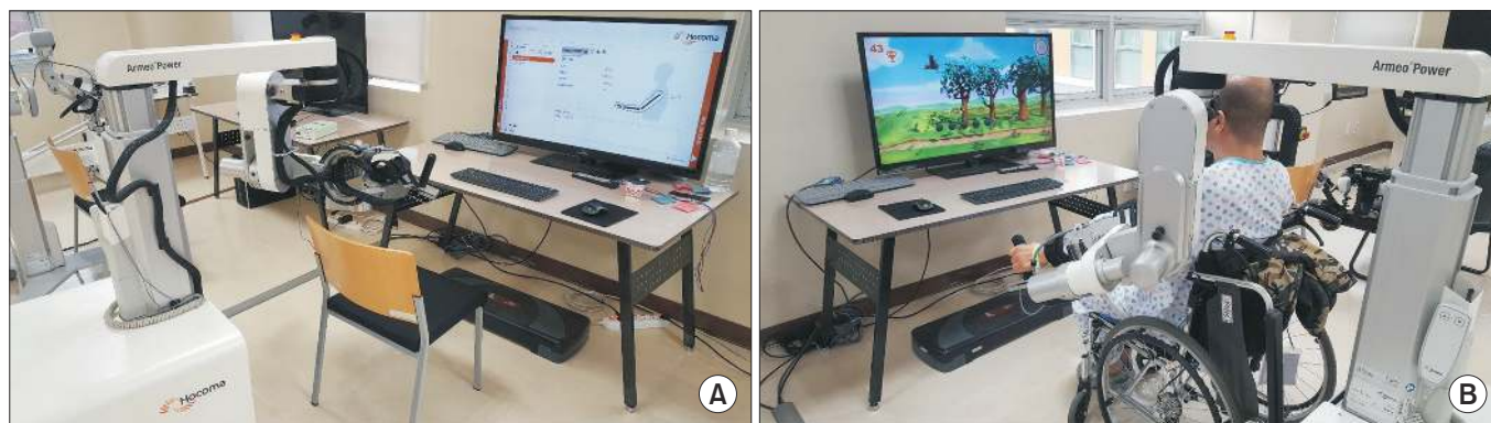
Fig. 1. (A) ArmeoPower, a rehabilitation exoskeleton that mainly trains proximal upper limb including shoulder, elbow, and wrist. (B) The patient training proximal upper limb with ArmeoPower.
