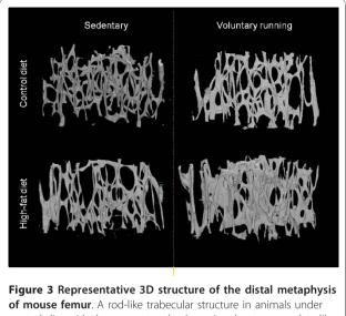
of mouse femur. A rod-like trabecular structure in animals under control diet with the access to wheel running, but a more plate-like structure in HFR animals was found.
