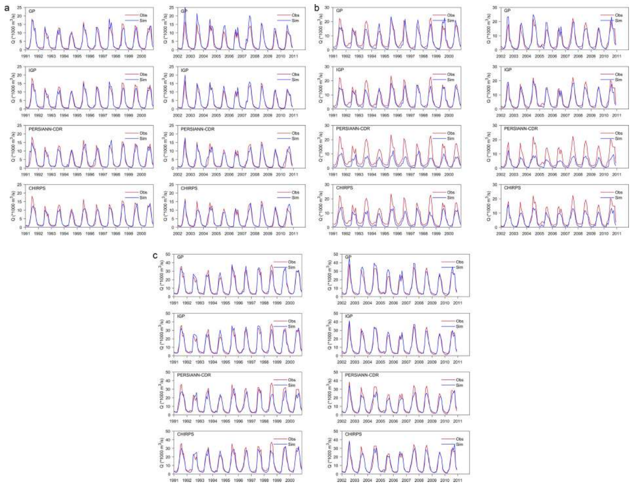
Fig. 5. Comparison of simulated and observed monthly stream flow of best simulation at a) Monywa b) Sagaing and c) Pyay during Calibration (1991–2000) and Validation (2002–2010) periods.
