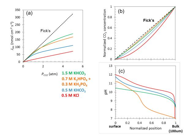
**Figure 3.** (a) Model results (assuming 100% conversion of  $CO_2$  to  $CH_4$ ) of  $CO_2$  pressure dependence of  $J_{lim}$  in 4 different electrolytes; the dotted line indicates assuming Fick's law. (b)  $CO_2$  concentration and (c) pH within the 100 µm boundary layer at  $P_{CO2}$  of 2 atm.
