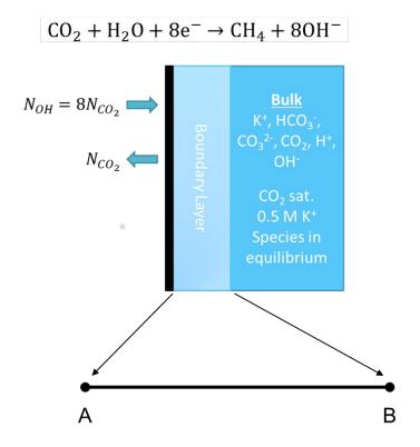
**Figure 1.** Schematic illustration of 1-D simulation model assuming 100%  $CH_4$  faradaic efficiency
