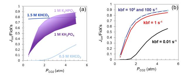
**Figure 7.** Comparison of pressure dependence of  $J_{lim}$  for (a) 0.5 and 1.5 M KHCO<sub>3</sub> and a range of 1 M phosphate from  $K_2HPO_4$  to  $KH_2PO_4$  (purple area) and (b) as a function of phosphate buffer kinetic rates (see equation 4) using 1 M  $K_2HPO_4$ . All simulations done assuming 90 mA/cm<sup>2</sup> total current density.
