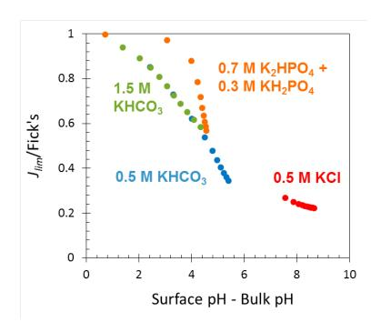
**Figure 4.** Relationship between normalized  $J_{lim}$  (to that expected from Fick's law) and pH change within the boundary layer for 4 different electrolytes.
