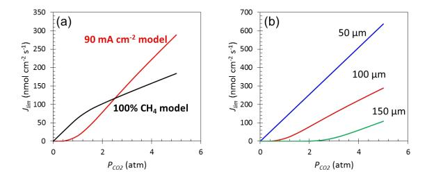
**Figure 6** (a) Comparison of pressure dependence of  $J_{lim}$  between 100% CO<sub>2</sub> reduction and constant OH<sup> $\square$ </sup> flux (corresponding to 90 mA cm<sup>-2</sup>) models with the phosphate buffer solution and 100 μm boundary-layer thickness. (b) The effect of boundary-layer thickness on the pressure dependence of  $J_{lim}$  using the constant OH<sup> $\square$ </sup> flux model with phosphate buffer solution.
