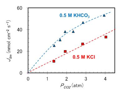
**Figure 2.**  $CO_2$  pressure ( $P_{CO2}$ ) dependence of limiting rate of mass transport of  $CO_2$  ( $J_{lim}$ ) in 0.5M KHCO<sub>3</sub> (blue triangles) and 0.5M KCl (red squares) solutions (dotted lines are guides for the eye only).
