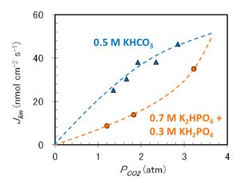
**Figure 5.** Experimental results of  $P_{CO2}$  dependence of  $J_{lim}$  in 1 M phosphate buffer (orange circles) compared to 0.5 M KHCO<sub>3</sub> (blue triangles).
