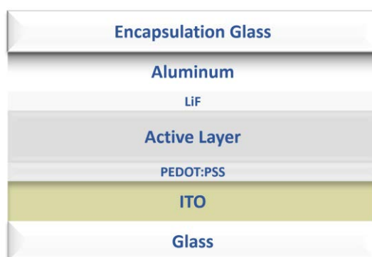
Figure 7. Conventional OSC device architecture. Incoming photons enter the device from the bottom semi-transparent ITO contact and are reflected by the top Al contact.
