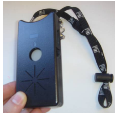
Figure 2: Sociometric badges can capture group dynamics in real-time. It is intended to be worn around one's neck.
