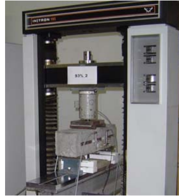
Fig. 2. Bending test setup.
