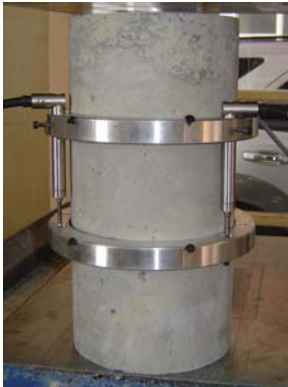
Fig. 1. Compressive test setup.
