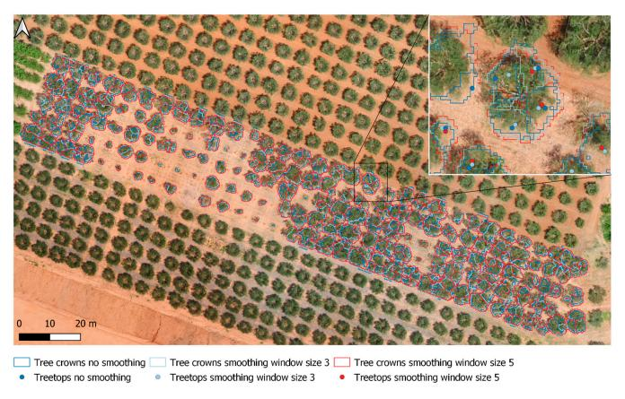
**Figure 5.** The results of the ITD approach applied to olive trees. Due to the specific canopy shape of the olive trees, individual branches were falsely identified as individual trees.
