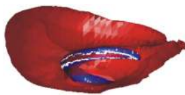
Fig. 20 Reconstructed HVC ( \bar{\omega}_z^{ap} = 5000 \text{ s}^{-1} ) and flame surface density ( \overset{\leftrightarrow}{\Sigma}^{ap} = 0.12 \text{ mm}^{-1} ) for flame 3 at \phi_a = 3 ( p = p_{\min} ). The HVC was below the flame when axially contracted.
