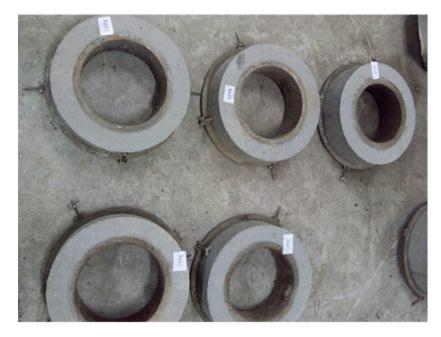
Figure 2. The picture of the restrained concrete ring test.
