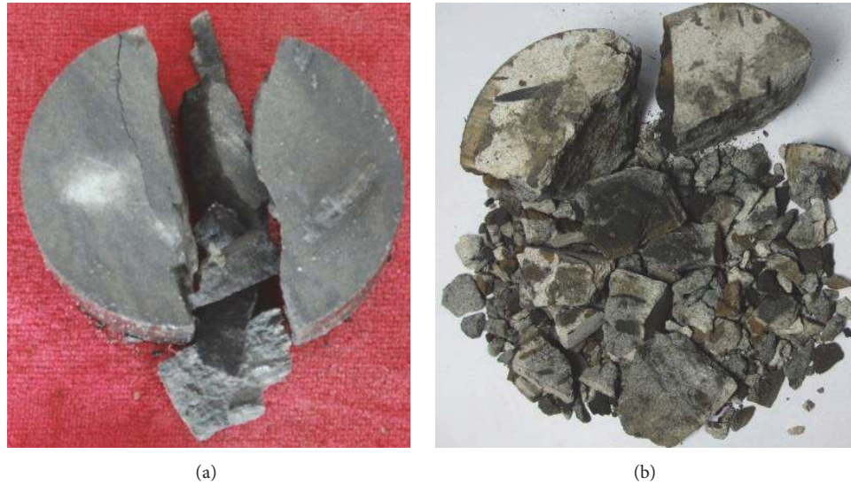
FIGURE 7: Dynamic Brazilian disc experiment specimen destruction: (a) normal temperature; (b) after 800°C heat treatment.
