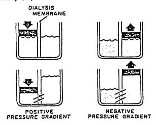
Fig. 3-5. Ultrafiltration. (Adapted from Nosé, Y.: Manual on artificial organs, Vol. I: The artificial kidney, St. Louis, 1969, The C. V. Mosby Co.)
