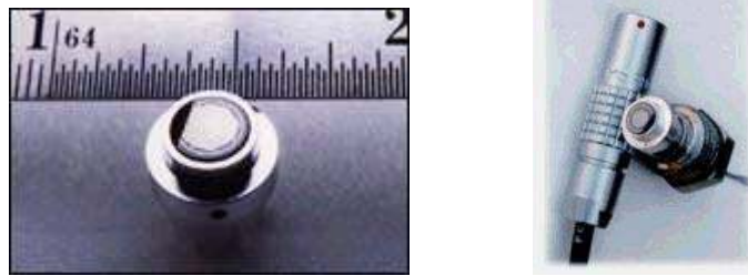
Figure 2.6a. Vatell HFM-7 Heat Flux Microsensor Source: Vatell Corporation website
