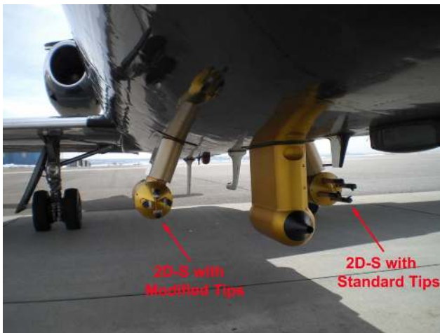
Fig. 3. Photograph showing the SPEC Learjet used in the SPARTICUS project with two 2D-S probes, one with tips modified to reduce shattering, and the other with standard tips.
