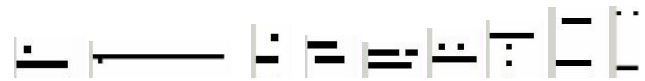
Fig. B1. Examples of line plus dot patterns caused by noisy photodiodes.
