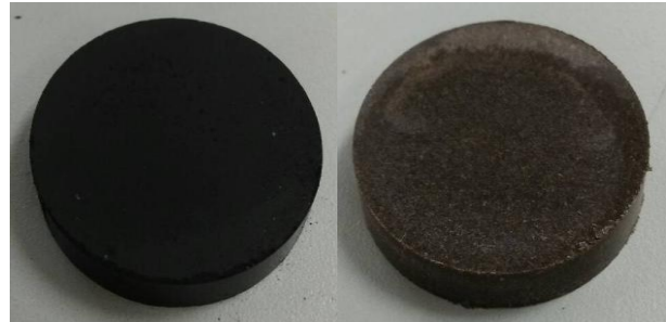
Fig. 3 Pallet sample of POFA (left) and BSP (right)
