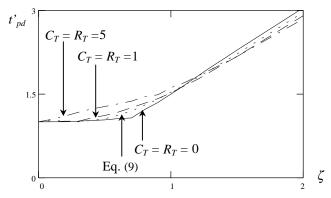
Fig. 2. Comparison of the accuracy of (9) to AS/X [14] simulations of the time scaled 50% propagation delay  $t'_{pd}$  of an *RLC* transmission line with a source resistance  $R_{tr}$  and a load capacitance  $C_L$ . The propagation delay is plotted versus  $\zeta$  for different values of  $R_T$  and  $C_T$ .
