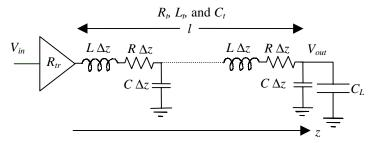
Fig. 1. A CMOS gate driving an RLC transmission line.
