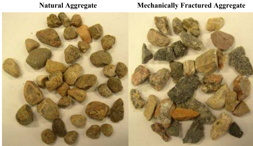
Figure 2.9 Effect of Mechanical Crushing on Aggregate Shape
