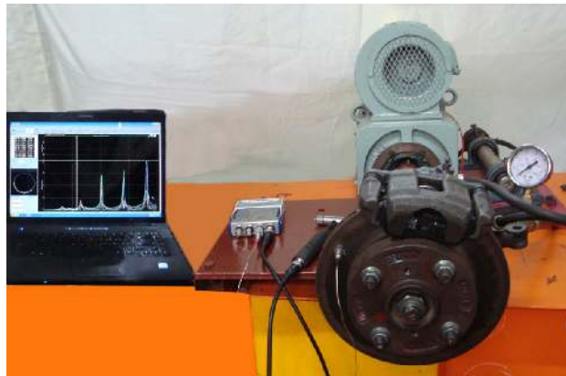
Figure 4: Experimental modal analysis of brake assembly.
