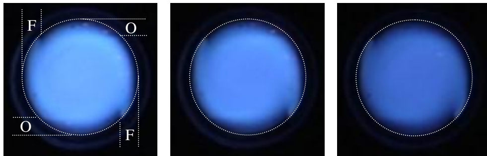
Fig. 3.16 Appearances of methane/oxygen flames ( W=2 mm, L=50 mm, Q_{\text{CH}_4} = 1.0 \text{ m}^3_{\text{N}}/\text{h} , Q_{\text{O}_2} = 5.0 (left), 6.0 (center), 8.0 (right) \text{m}^3_{\text{N}}/\text{h} ).
