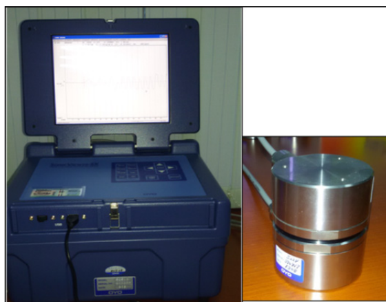
Figure 1. The equipment for ultrasonic measurement
