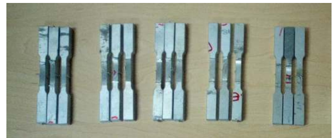
Fig. 3. Tensile samples evaluated.
