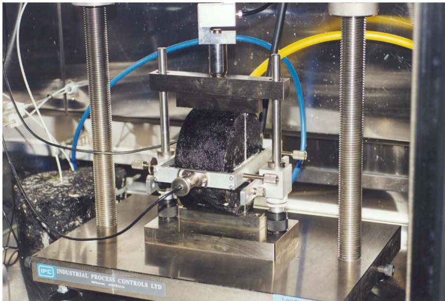
Figure 2: Resilient modulus test
