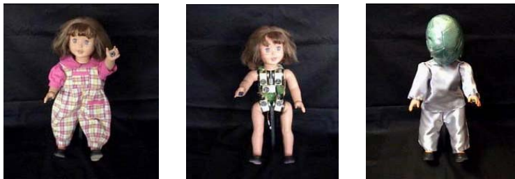
Figure 1. The robot in its two different appearances (the centre figure shows the 'undressed' version revealing the robotic parts that control its movement)
