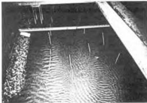
Fig. 10 The sand ripples under the short-crested wave which did not break.
