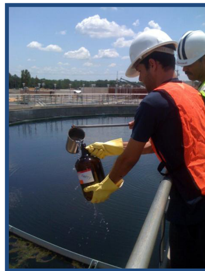
Figure 4: Obtaining samples from a secondary clarifier at the Thomas P. Smith Water Reclamation Facility, Tallahassee, FL.
