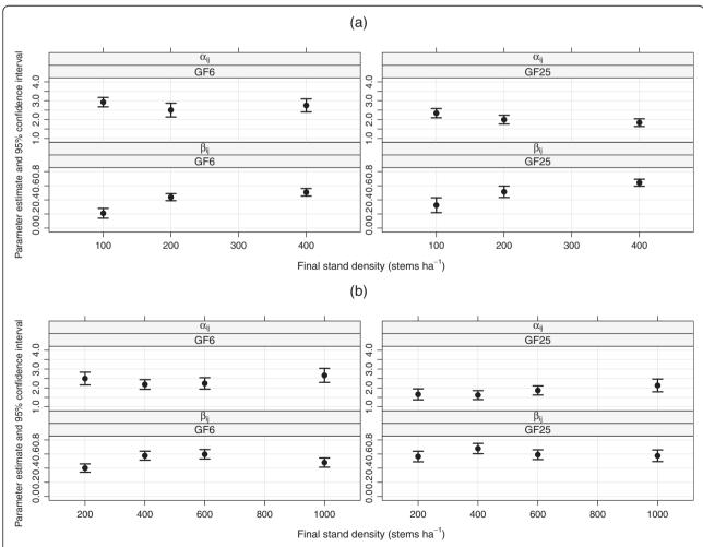
Figure 6 Plots of Equation [3] fixed parameter estimates and 95% confidence intervals for the breast height ring level modulus of elasticity trends for GF6- and GF25-rated trees at various final stand densities in (a) the pruned experiment; and (b) the unpruned experiments.
