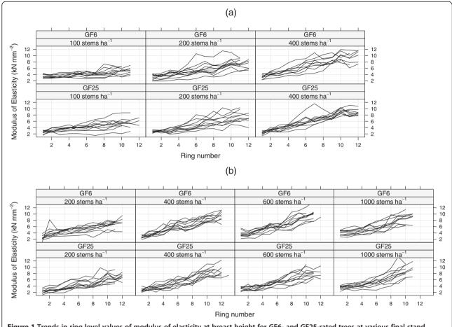
Figure 1 Trends in ring level values of modulus of elasticity at breast height for GF6- and GF25-rated trees at various final stand densities in (a) the pruned experiment; and (b) the unpruned experiment.
