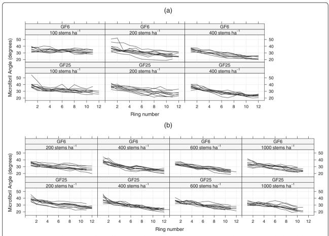
Figure 4 Trends in ring-level values of microfibril angle at breast height for GF6- and GF25-rated trees at various final stand densities in (a) the pruned experiment; and (b) the unpruned experiments.
