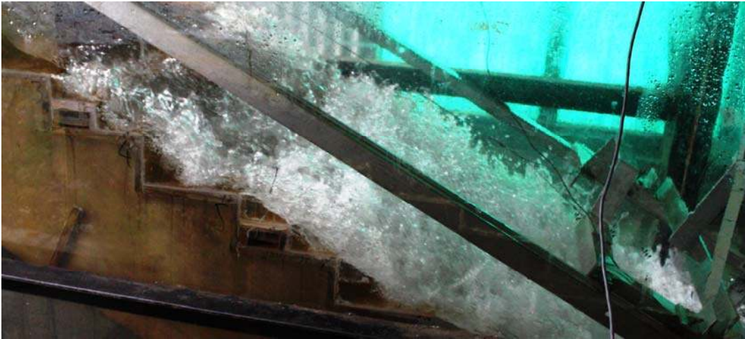
(a) Transition flow regime: d_c/h = 0.78 , q_w = 0.069 \text{ m}^2/\text{s} , R = 2.7 \times 10^5 ; note the trolley for the double-tip conductivity probe in the right bottom corner
