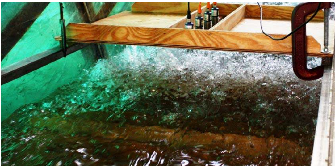
(b) Free-surface waves and fluctuations in the skimming flow regime: d_c/h = 1.46 , q_w = 0.175 \text{ m}^2/\text{s} , R = 6.9 \times 10^5 ; wooden support with the acoustic displacement meters above the air-water flows
