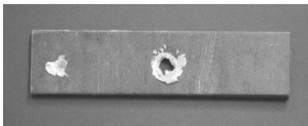
5 Blow-through hole of AR-B condition
