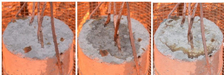
Figure 11. Water migration/bleeding on top of the specimen surface.
