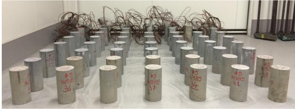
Figure 4. Test specimens in the controlled room of 27°C and 70% relative humidity.
