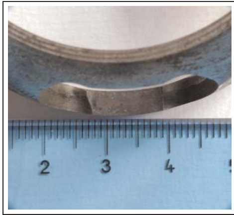
Figure 2. Wear due to contact between the ball and the cage in an automotive Rzeppa joint after functioning for 5000 h.
