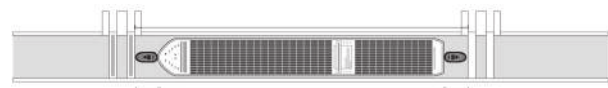
Figure 4 – Layout of a lock in the expanded Canal with the location of the double sliding gates and the tugs in position [8]
