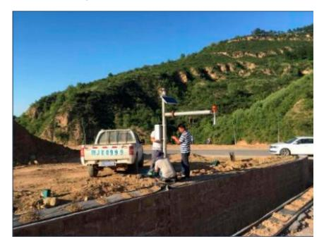
Figure 4. The auto-recording tipping bucket rain gauge and radar water level sensor at watershed outlet.
