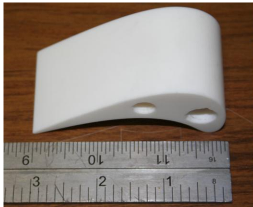
Figure A.1 Macor tip of the test blade
