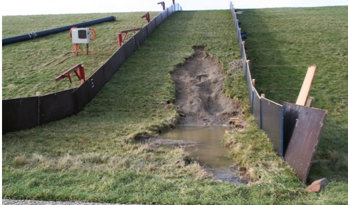
Figure 3.5 Geometrical transition (at toe of dike)
