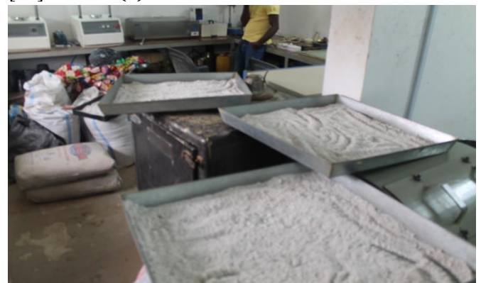
Figure 1. Showing RHA being Dried and Processed in the Laboratory.
