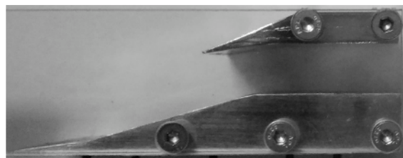
(a) A photographic view of the uncontrolled Mach 2.2 intake developed for the present study
