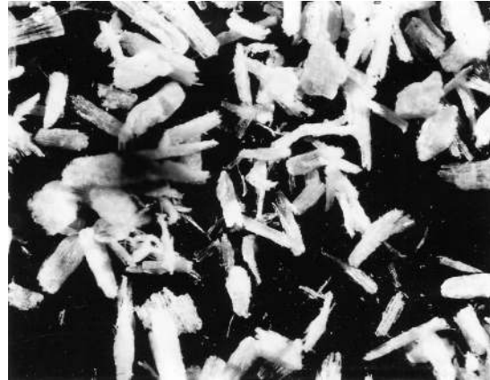
FIG. 3. Commercial 40-mesh wood flour.
