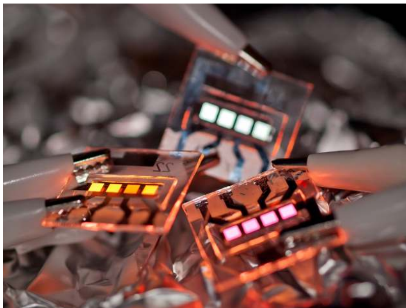
Figure 1.1: Photograph of three different OLEDs employing multiple emitters. While each OLED consists of the same materials, the different color is produced by varying the microcavity of the thin-film layer stack.
