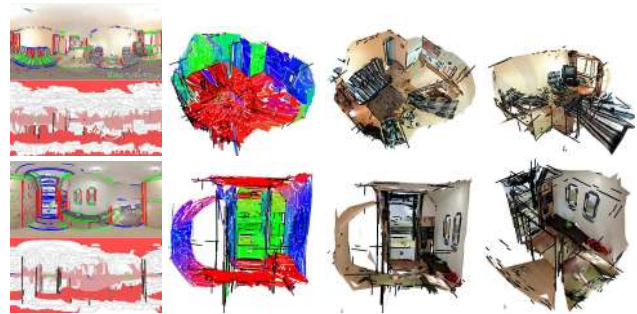
Figure 14: Two failed cases. In the first case, the reconstruction is misled by the false horizontal superpixels that cover the sofa in the room. In the second case, some wall superpixels are incorrectly identified as parts of the floor, which leads to a false illusion of doors open on the wall.
