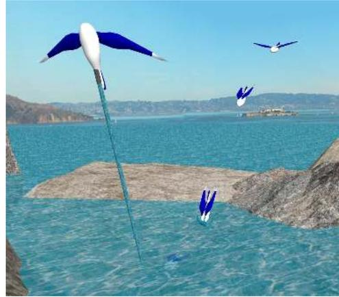
Fig. 1: Concept sketch of an Aquatic Micro Aerial Vehicle diving into the water, gathering data and retaking flight.
