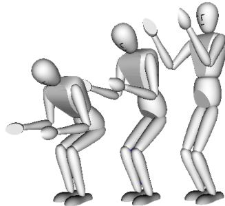
Figure 2. Posture Behavior: a sequence of snapshots from the dynamic simulation of a 21-degree-of-freedom humanoid system. The hands are haptically teleoperated, while the remaining degrees of freedom are controlled automatically in the posture space. The posture controls the center of mass to balance the robot, while maintaining a natural arm configuration.
