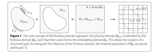
On  $\Gamma_N$  of the physical domain, the traction vector t specifies the Neumann boundary conditions.
