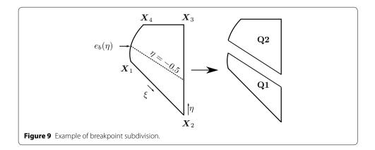
decomposition: all cells that are bounded by piecewise defined curves are further subdivided along the breakpoints of the curves.
