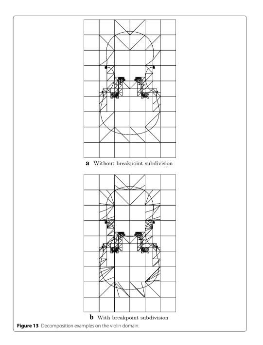
direction in each cell. If the breakpoints are not taken into account as explained in "Piecewise definition of the boundary", the error remains higher regardless of how many integration points are distributed in the cells. However, if the integration cells are subdivided along the breakpoints of the bounding curves, the error in the energy norm converges to machine precision.
