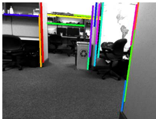
Fig. 5: Top: The 3D trajectory of the IMU-camera pair during the experiment. The Std-VINS erroneously treats rotations around gravity as observable, which results to a rotated trajectory. Bottom: Representative camera image from the experimental dataset with the extracted straight line edges superimposed (best viewed in color).
