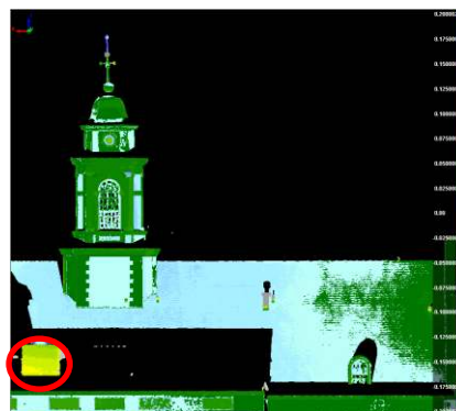
Figure 1. Deviation patterns color coded for a roof of a building: in the circle at the bottom left, an object has larger deviations (yellow) compared with the other parts of the roof (blue and green). Such deviation patterns can guide engineers to investigate and analyze that part of the model and data in depth.
