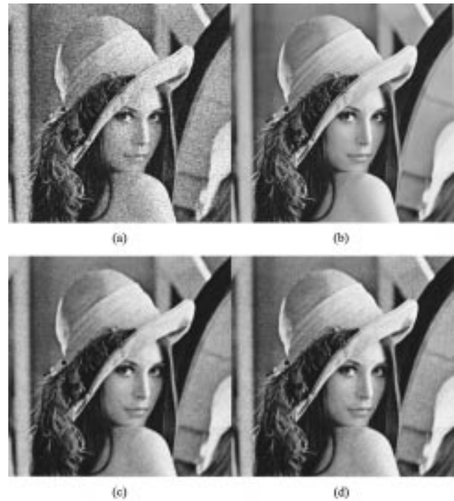
Fig. 15. Comparison of image quality between the output image of the NF trained to reduce quantum noise in natural images and that of its approximate filter. (a) Noisy input image. (b) Teaching image. (c) Output image of the trained NF. (d) Output image of the approximate filter.
