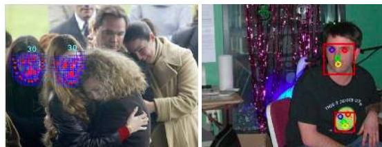
Figure 1. Hard cases under uncontrolled environment: extreme poses could lead to missed detections while cluttered background could lead to false detections.
