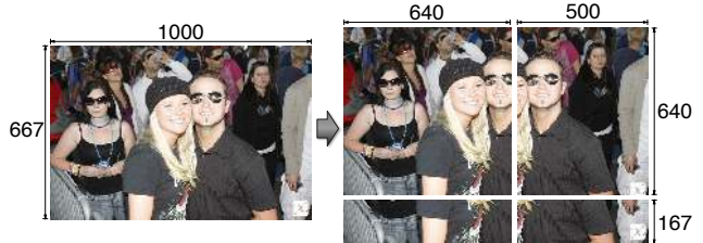
Figure 7. Large image is divided into overlapped tiles for memory constrained detection
