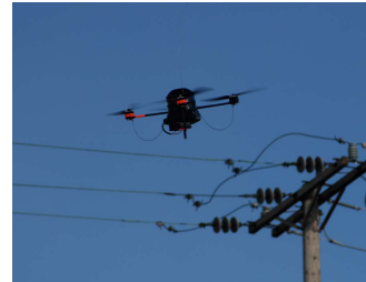
Fig. 1. The autonomous quad-rotor aerial vehicle used for testing. Here, the vehicle is close to a typical pole and wire obstacle in the environment. The system is equipped with a computer, a GPS, an inertial measurement unit, and a lidar scanner to sense the environment. The size of the vehicle with rotors is less than one meter.
