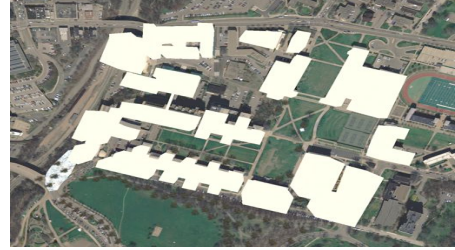
Fig. 5. The virtual campus environment of Carnegie Mellon University, Pittsburgh, PA that is used in the simulation experiments. Buildings that were added to the digital elevation model are shown in white. A hemispherical 200m range 3D range sensor is simulated to update the environment map held by the robot.
