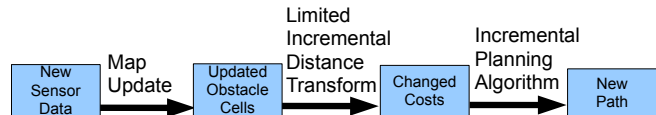
Fig. 2. Data flow in a completely incremental planning paradigm. Sensor data causes an update to the environment map which propagates to changes in the cost function used by the planner. Finally an incremental path planner calculates a new path to the goal with the changed cost values.
