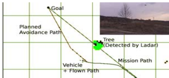
Fig. 9. This sequence of images shows our autonomous quadrotor micro aerial vehicle (Fig. 1) avoiding a tree that is in the straight line mission path to its goal. As soon as the robot detects the obstacle it plans a path in 3D with a wide berth around the obstacle. The cost function is set up in such a way that the robot will prefer to move laterally and therefore we only show a top view. Since d_{max} = 11 the obstacle is avoided by a large margin. The mission path is shown in black and the planned avoidance path is shown in red. The black line shows the path of the vehicle as recorded by GPS. The tree obstacle is shown in green.
